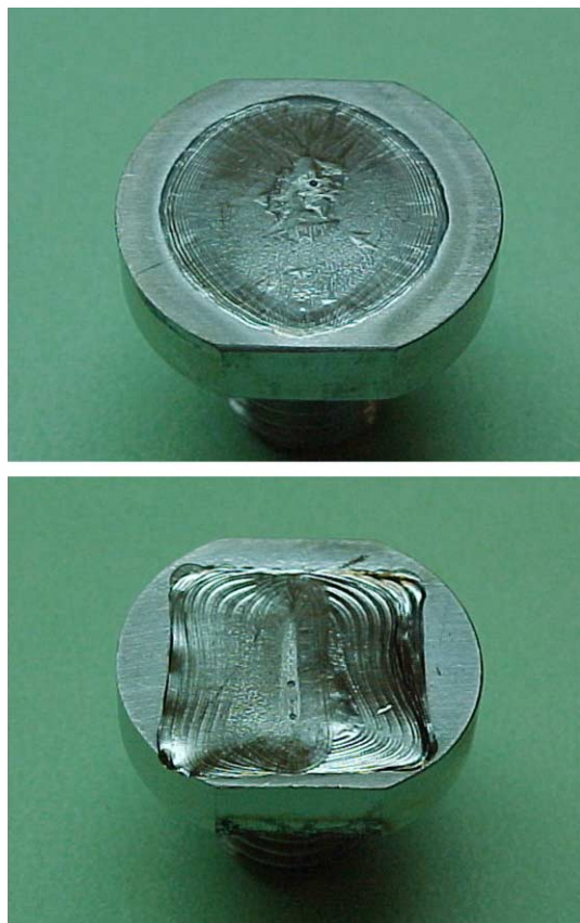
Fig. 19. As-welded specimens of 316LN. Top: TIG weld. Bottom: automated electron beam weld. In all cases, the substrate condition was annealed 316LN with an as-machined surface.
